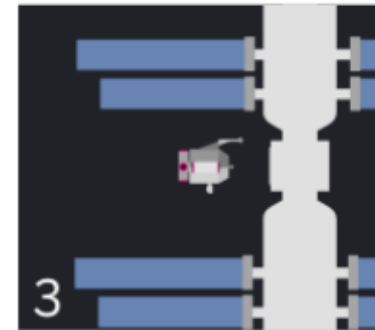
Thrusters cause pod to move in opposite direction OR pod hits space station and bounces off.
