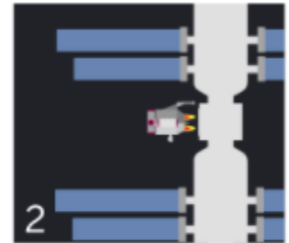
2 Thrusters fire to stop the pod.
