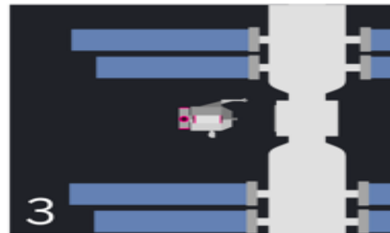
Thrusters cause pod to move in opposite direction OR pod hits space station and bounces off.
